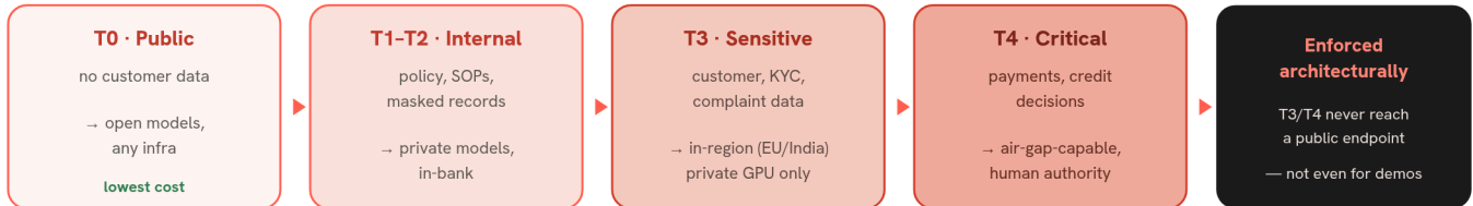
Figure 5 — T0-T4 data-class routing: the gateway sends each request to the right model and infrastructure for its sensitivity — the most sensitive classes are architecturally barred from public AI.
